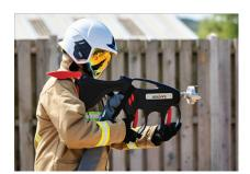
Fires can generate temperatures in excess of 600°C. The use of high pressure water mist produces a rapid reduction in temperature to less than 100°C after a short period of time enabling safer access to the fire zone by firefighting personnel.
